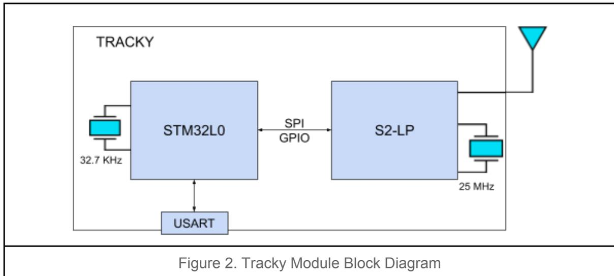
Figure 2. Tracky Module Block Diagram
